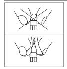
This fixture is fitted with a discharge lamp which is highly susceptible to damage if improperly handled. Never touch the lamp with your bare fingers as the oil from your hands will shorten lamp life. Also, never move the fixture until the lamps have had ample time to cool. Remember, lamps are not covered under warranty conditions.
