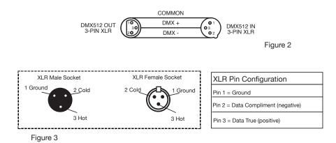
**Special Note: Line Termination.** When longer runs of cable are used, you may need to use a terminator on the last unit to avoid erratic behavior. A terminator is a 90-120 ohm 1/4 watt resistor which is connected between pins 2 and 3 of a male XLR connector (DATA + and DATA -). This unit is inserted in the female XLR connector of the last unit in your daisy chain to terminate the line. Using a cable terminator (ADJ part number Z-DMX/T) will decrease the possibilities of erratic behavior.
