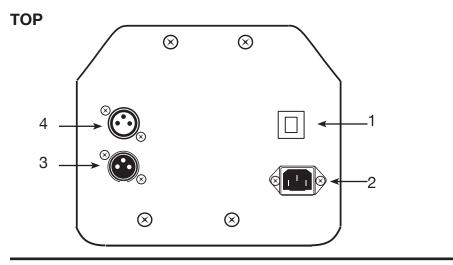
**1. Breaker -** A 5A built-in safety breaker to reduce the risk of electrical shock or fire and protect the circuitry. In the case of a internal short or power surge.
