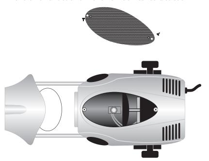
Remove the lamp from the socket and insert a new one as illustrated above.
