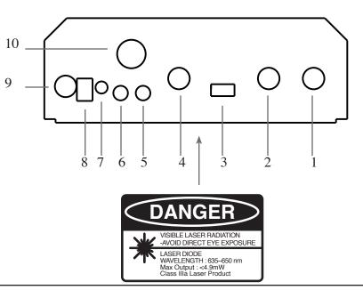
**1. Pattern Knob 2** - This knob, when adjusted, generates different patterns when in manual mode.
