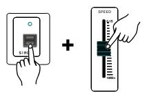
(3) Press the "STROBE" button again to disengage the strobe effect.
