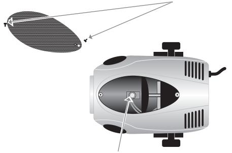
Remove the lamp from the socket and insert a new one as illustrated above.
