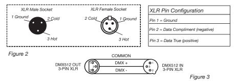
**Special Note:** Line Termination. When longer runs of cable are used, you may need to use a terminator on the last unit to avoid erratic behavior. A terminator is a 90-120 ohm 1/4 watt resistor which is connected between pins 2 and 3 of a male XLR connector (DATA + and DATA -). This unit is inserted in the female XLR connector of the last unit in your daisy chain to terminate the line. Using a cable terminator (ADJ part number ZDMX/T) will decrease the possibilities of erratic behavior.
