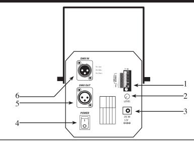
**1. Dipswitches -** These switches serve two functions. In master-slave mode these switches are used to assign a specific head address. In DMX mode these switches are used to assign a DMX address to the unit. In DMX mode each switch corresponds to a specific value based on binary code. See page 7 for a detailed explanation of DMX binary code.
