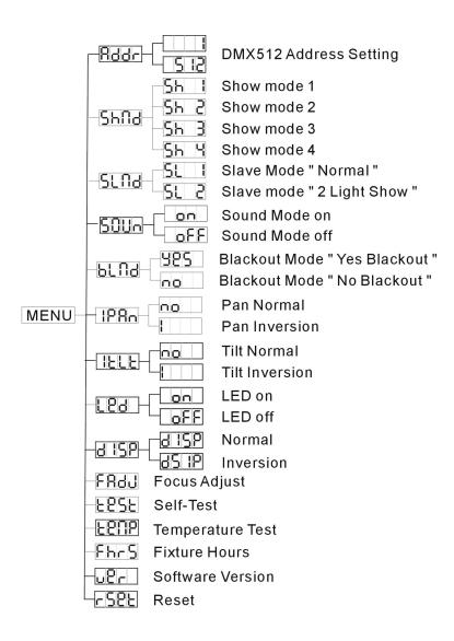
System Menu: When making adjustments you can press ENTER to confirm your setup or you can wait 8 seconds for automatic setup. To exit without making any adjustments press the MENU button.
