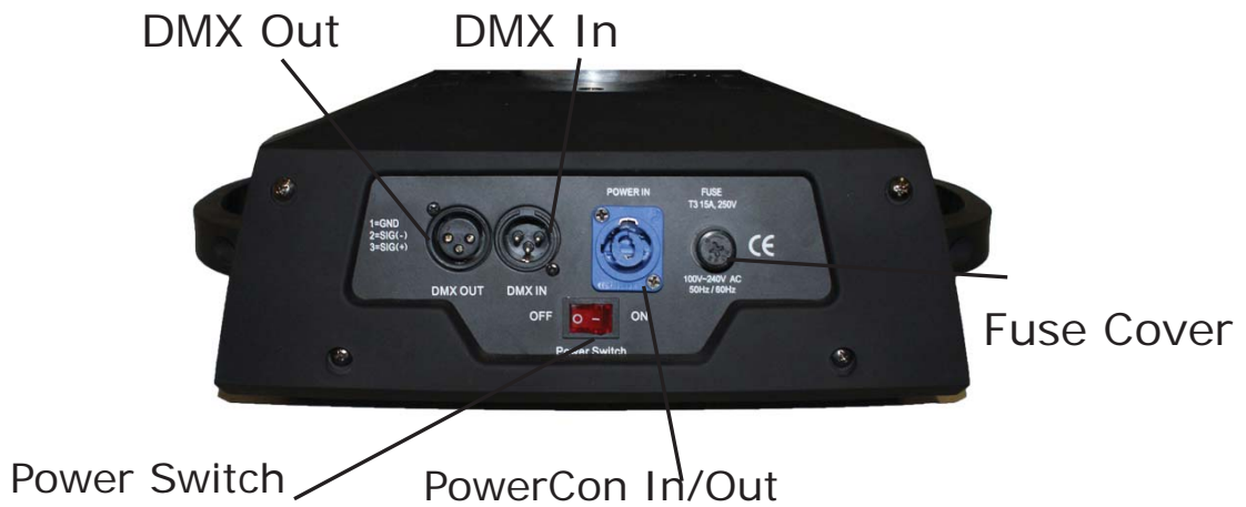
Figure 2: The Rear Connections
