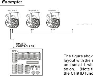
The figure above shows a simple DMX512 layout with the starting address of the first unit set at 1, with the second set at 10 and so on... (Note that when used in this way, the CH9 ID function must be inactive (CH9=0))
