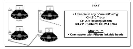
Once the heads have been linked correctly, as shown, then it is necessary to select th appropriate channel for each head. On the rear of each 'linkable' unit you will find a rotal selector which has positions 1 to 4 clearly marked.
