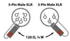
The terminator plug connects to the DMX Out socket of the last DMX fixture in the daisy chain.
