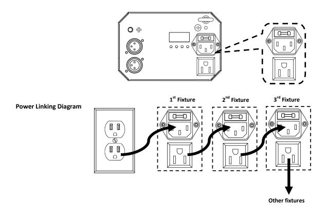
You can power link up to 24 DMF-10 units on 120 VAC or up to 44 DMF-10 units on 230 VAC.
