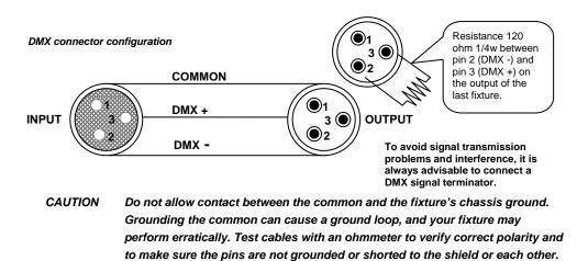
Cabling must have a male XLR connector on one end and a female XLR connector on the other end.
