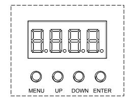
The Control Panel shows the current state of the unit. It is used to select the operating mode, as well as the sub-features. For a detailed layout of the control panel functions, please see the "menu map" section on the following page.
