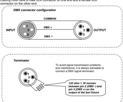
Cabling must have a male XLR connector on one end and a female XLR
