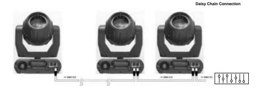
If this is your first time addressing a fixture using the DMX-512 control protocol than I suggest jumping to the Appendix Section and read the heading "DMX Primer". It contains very useful information that will help you understand its use.
