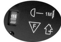
Figure 1 - AC Voltage Switch
