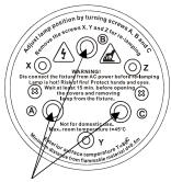
Lamp Alignment Screws, A, B & C
