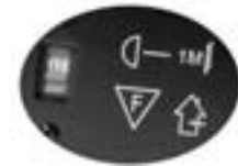
Figure 1 - AC Voltage Switch
