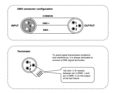
Cabling must have a male XLR connector on one end and a female XLR connector on the other end.
