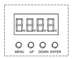
The Control Panel shows the current state of the unit. It is used to select the operating mode, as well as the sub-features. For a detailed layout of the control panel functions, please see the "menu map" section below.
