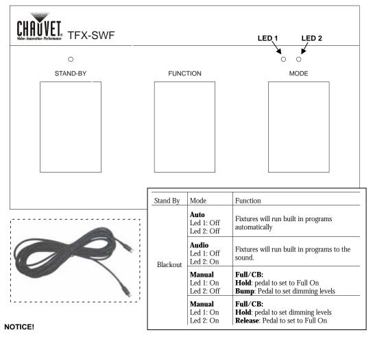
The TFX-SWF Foot Controller is used only in master/slave mode. Connect the 8-pin connector of the foot controller into its respective connector on the first unit in the daisy chain. The table below describes the functions of the TFX-SWF Controller.
