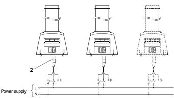
After all the operations described above have been carried out, supply power to the device and check that the lamp lights up, and that bubble production and the rotation of the colour disc begin.
