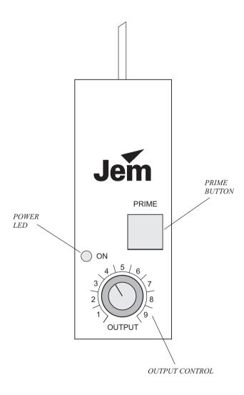
The Technohaze comes with a compact remote allowing the user to prime the pump and control the output level.
