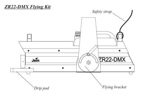
The ZR22-DMX flying kit enables the machine to be fixed to rigging and ceilings for use where the ZR22-DMX is best situated in a flying position. The Kit has everything you need to give maximum safety and reliability when fixing to rigging etc. The kit comes with full fixing instructions. The kit even includes a drip pad for catching unwanted drips that can occur when smoke machines are angled down.
