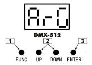
In the MODE OPTION setting, the stand alone laser show that you are going to choose is flashing. Press UP or DOWN to change stand alone laser show, you will have 8 different stand alone preprogrammed laser show. Their DISPLAY and EFFECT are listed below:
