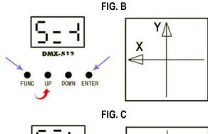
Using the up/down buttons, set the LED display to match Fig. C. This will flip the graphic in the Y direction.
