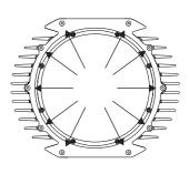
7. Cross-tighten the Allen screws with a torque of 3 N.m (2.2 Ft-Lbs). With this torque, the seal will be compressed by about one-third.
