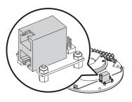
by inserting a an RJ-45 termination plug (for example an 100 ohm RJ-45 ISDN terminator) into the DMX data output of the last J-Box.
