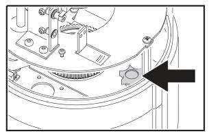
4 Remove the gobo plate from the fixture.
