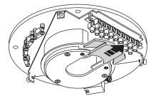
3 Pass the cables and mounting flange of the Imager though the center of the J-Box cover.
