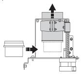
4 Slide the optional lens in under the standard lens, and screw it to the thread on the standard lens.
