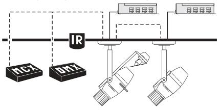
The J-Box is connected to a controlling device and power. An Imager Base supplies power to the Imager (via the J-Box).
