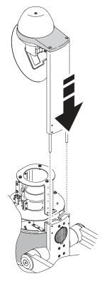
13 Place the cable so that it stays out of the optical path.
