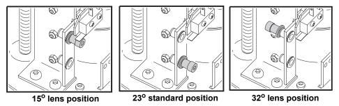
Note that for the 32 degree lens the pin is removed and inserted from the other side of the plate.
