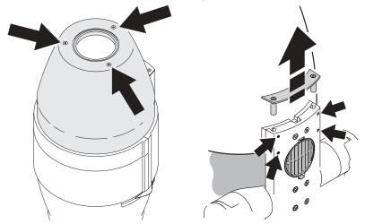
9 Using a 2mm Allen wrench, loosen the 4 recessed Allen screws on the spine of the fixture and remove the cover plate.
