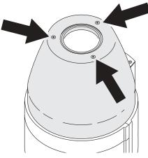
3 Unscrew the thumb screw holding the gobo plate in place.
