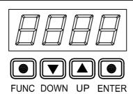
Projector configuration can be set conveniently via pressbutton switch and digital display. Turn the projector on and the digital display will show DMX address you set and save last time and it can be reset and saved again as you please.
