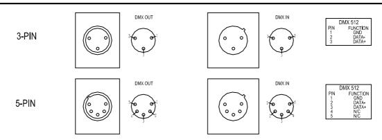
Connection between controller and projector and between one projector and another must be made with 2 core-screened cable, with each core having at least a 0.5mm diameter. Connection to and from the projector is via cannon 3 pin (which are included with the projector) or 5 pin XLR plugs and sockets. The XLR's are connected as shown in the figure above.
