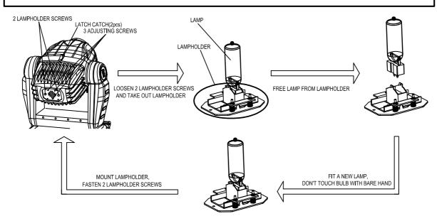
Lock tilt before fitting/replacing the lamp.
