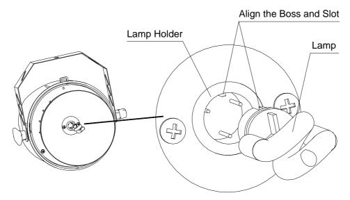
First, remove the front cover and then plug the lamp into the lamp-holder. When installing, hold the screw part of the lamp and let the slot of the lamp align the boss of the lamp-holder before plug the lamp completely.
