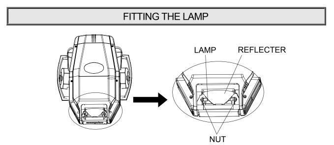
Lock the yoke before fitting/replacing the lamp.
