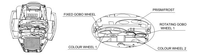
Disconnect the fixture from power. Lock Tilt. Carefully lift off the cover by undoing the 6 screws.
