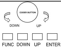
Projector configuration can be set conveniently via pressbutton switch and LCD display. Turn the projector on and the LCD display will show DMX address you set and save last time and it can be reset and saved again as you please. Launch the projector. Press button ENTER more than 5 seconds to unlock panel.
