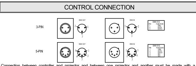
Connection between controller and projector and between one projector and another must be made with a 2 core-screened cable, with each core having at least a 0.5mm diameter. Connection to and from the projector is via cannon 3 pin (which are included with the projector) or 5 pin XLR plugs and sockets. The XLR's are connected as shown in the figure above.
