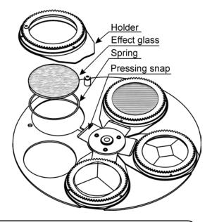
CAUTION! The effect glass holder with the magnet must be placed in the same glass position as it was placed before glass replacement!
