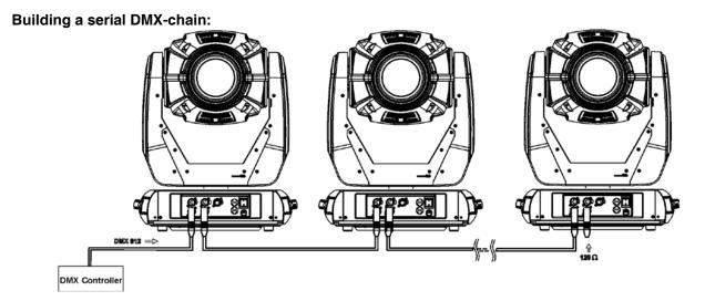
Connect the DMX-output of the first fixture in the DMX-chain with the DMX-input of the next fixture. Always connect one output with the input of the next fixture until all fixtures are connected.
