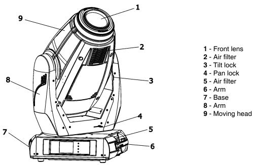
The head should be locked for transportation- the tilt lock latch (2) and the pan lock latch (3) have to be in the locked positions. To unlock the head, move these latches to unlock positions before operating the fixture.
