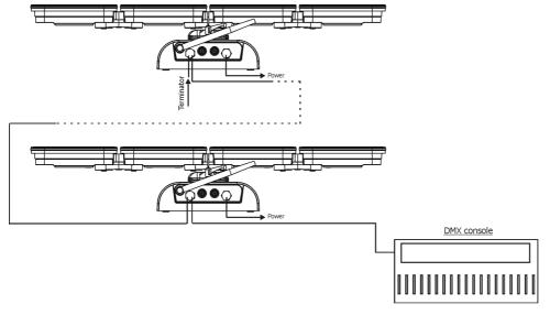
Caution: Terminate the link by installing a termination plug in the output of the last fixture. The termination plug is a male 3-pin XLR plug with a 120 Ohm resistor soldered between Signal (–) and Signal (+).
