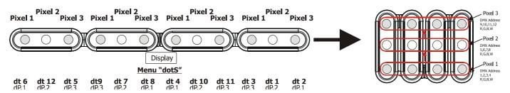
Only DMX channels 1-12 are used for control this pixel configuration. If all pixels have the same pixel position, the fixture will behave as one pixel.
