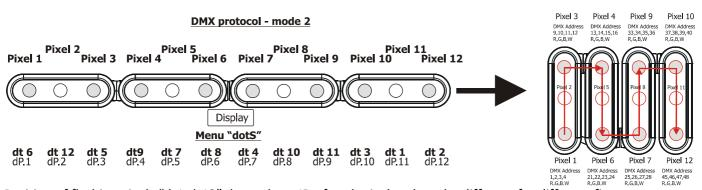
Position of flashing pixels "dt1-dt12" depends on ID of each pixel and can be different for different fixtures.
