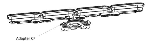
If the LED modules and the base are installed separately on the metal structure (LED modules and the base are galvanic interconnected), the LED modules fall under protection class I and must be grounded in accordance with all national and local electrical and construction regulations.
